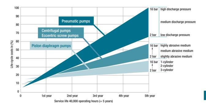
The costs of wear parts and energy are low for piston diaphragm pumps compared to other types of pump.
